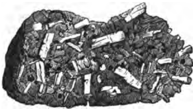
FIG. 30.—A piece of granite, showing the composition of a Crystalline Rock.
